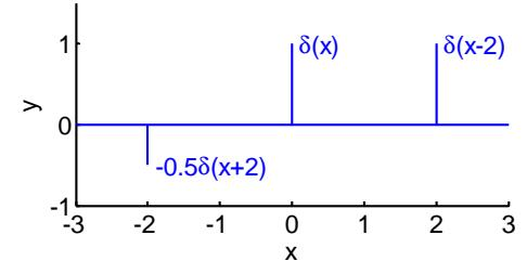
Amplitude Scaling:  $b\delta(x)$
