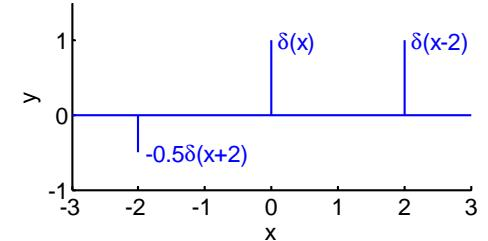
Amplitude Scaling:  $b\delta(x)$
