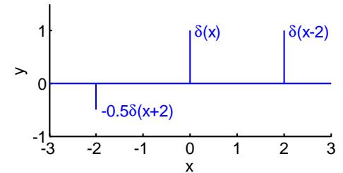
Amplitude Scaling:  $b\delta(x)$
