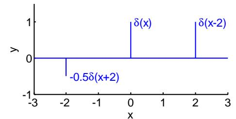
Amplitude Scaling:  $b\delta(x)$
