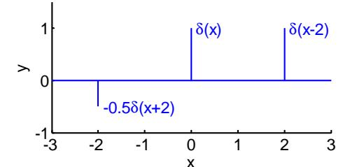
Amplitude Scaling:  $b\delta(x)$
