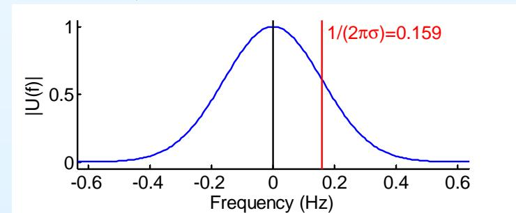
Uniquely, the Fourier Transform of a Gaussian pulse is a Gaussian pulse.
