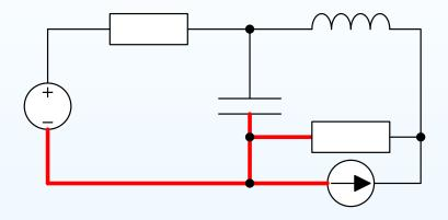
A *node* in a circuit is all the points that are connected together via the interconnecting wires. One of the four nodes in the diagram is coloured red. Assumption: Interconnecting wires have zero resistance so everywhere along a node has the same voltage.
