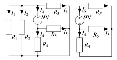
Much simpler - although none of the original currents  $I_1, \dots, I_5$  are now accessible. Current  $I_S$  and the three node voltages are identical.
