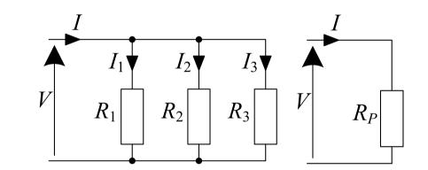
Replacing parallel resistors by their equivalent resistor will not affect any of the voltages or currents in the rest of the circuit.
