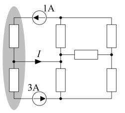
Note that here I ends up negative which means we chose the wrong arrow direction to label the circuit. This does not matter. You can choose the directions arbitrarily and let the algebra take care of reality.
