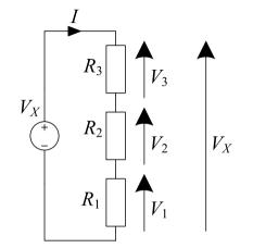
$V_X$  is divided into  $V_1: V_2: V_3$  in the proportions  $R_1: R_2: R_3$ .
