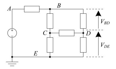
*Kirchoff's Voltage Law* (KVL) is a consequence of the fact that the work done in moving a charge from one node to another does not depend on the route you take; in particular the work done in going from one node back to the same node by any route is zero.
