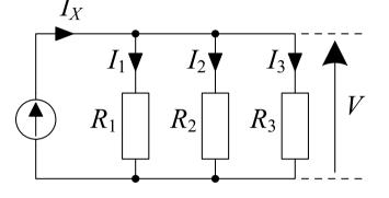
$$\frac{I_1}{I_X} = \frac{VG_1}{V(G_1 + G_2 + G_3)} = \frac{G_1}{G_1 + G_2 + G_3} = \frac{G_1}{G_F}$$
