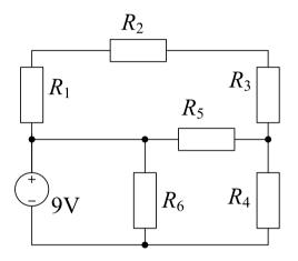
Parallel: Components that are connected to the same pair of nodes are said to be *in parallel*.
