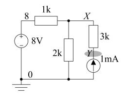
Ohm's law works OK if all resistors are in  $k\Omega$  and all currents in mA. (4) Solve the equations: X = 6, Y = 9 3: Nodal Analysis Aim of Nodal Analysis Nodal Analysis Stage 1: Label Nodes Nodal Analysis Stage 2: KCL Equations **Current Sources** Floating Voltage  $\triangleright$  Sources Weighted Average Circuit Digital-to-Analog Converter Dependent Sources Dependent Voltage Sources Universal Nodal Analysis Algorithm Summary
