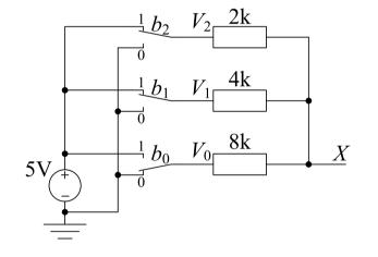
$$G_2 = \frac{1}{R_2} = \frac{1}{2} \text{ mS}, \dots$$
