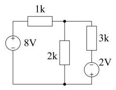
(1) Pick any node as the voltage reference. Label its voltage as 0 V. (2) If any fixed voltage sources are connected to a labelled node, label their other ends by adding the value of the source onto the voltage of the labelled end.
