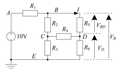
Ohm's Law:  $V_{BD} = IR_5$ KVL:  $V_{BD} = V_B - V_D$ KCL: Total current exiting any closed region is zero. 3: Nodal Analysis Aim of Nodal Analysis Nodal Analysis Stage 1: Label ▷ Nodes Nodal Analysis Stage 2: KCL Equations **Current Sources** Floating Voltage Sources Weighted Average Circuit Digital-to-Analog Converter Dependent Sources Dependent Voltage Sources Universal Nodal Analysis Algorithm Summary
