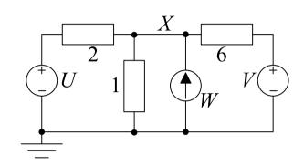
From the linearity theorem, we know anyway that X = aU + bV + cW so all we need to do is find the values of a, b and c. We find each coefficient in turn by setting all the other sources to zero:
