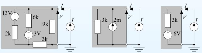
These four shaded networks are *equivalent* because the relationship between V and I is *exactly* the same in each case.
