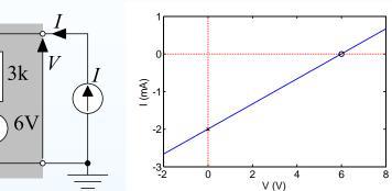
Open Circuit Voltage: If I = 0 then  $V_{OC} = V_{Th}$ . (X-intercept: o) Short Circuit Current: If V = 0 then  $I_{SC} = -\frac{V_{Th}}{R_{Th}}$  (Y-intercept: x)
