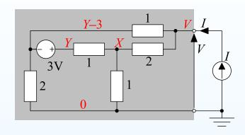
Step 1: Label ground as an output terminal + label other nodes.
