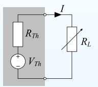
$$0 = \frac{dP_L}{dR_L} = \frac{(R_{Th} + R_L)^2 V_{Th}^2 - 2V_{Th}^2 R_L (R_{Th} + R_L)}{(R_{Th} + R_L)^4}$$
