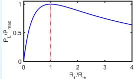
For fixed  $R_{Th}$ , the maximum power transfer is when  $R_L = R_{Th}$  ("*matched load*").
