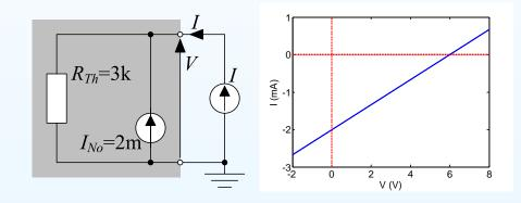
Open Circuit Voltage: If I = 0 then  $V_{OC} = I_{No}R_{Th}$ .
