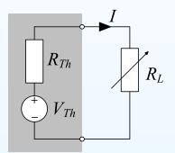
$$0 = \frac{dP_L}{dR_L} = \frac{(R_{Th} + R_L)^2 V_{Th}^2 - 2V_{Th}^2 R_L (R_{Th} + R_L)}{(R_{Th} + R_L)^4}$$
