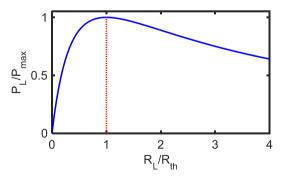
For fixed  $R_{Th}$ , the maximum power transfer is when  $R_L = R_{Th}$  ("matched load").
