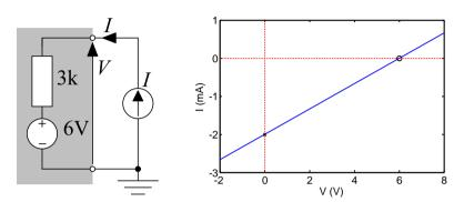
Open Circuit Voltage: If I = 0 then  $V_{OC} = V_{Th}$ . (X-intercept: o) Short Circuit Current: If V = 0 then  $I_{SC} = -\frac{V_{Th}}{R_{Th}}$  (Y-intercept: x)
