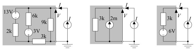
These four shaded networks are *equivalent* because the relationship between V and I is *exactly* the same in each case. The last two are particularly simple and are respectively called the *Norton* and *Thévenin* equivalent networks.
