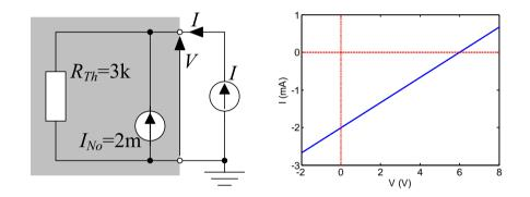
Open Circuit Voltage: If I = 0 then  $V_{OC} = I_{No}R_{Th}$ .
