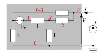
Step 1: Label ground as an output terminal + label other nodes. Step 2: Write down the equations (Y is a supernode)  $\frac{X-V}{2} + \frac{X}{1} + \frac{X-Y}{1} = 0$
