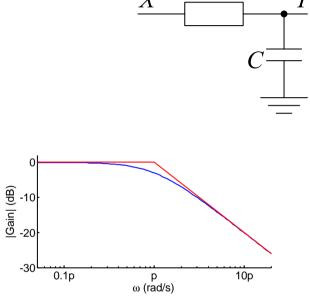
A *low-pass* filter because it allows low frequencies to pass but *attenuates* (makes smaller) high frequencies.
