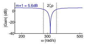
At  $\omega = p$ ,  $\left(\frac{j\omega}{p}\right)^2 = -1$ : numerator = zero resulting in infinite attenuation. The 3 dB notch width is approximately  $2\zeta p = 2(1-m)p$ .
