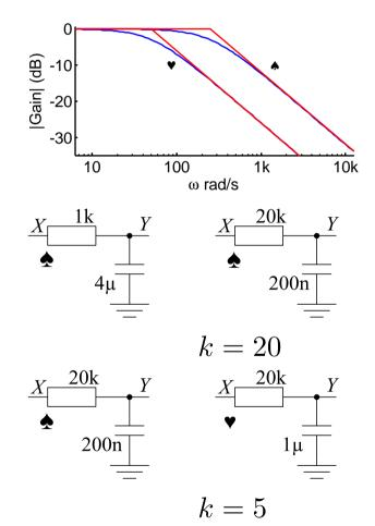
Must scale all reactive components in the circuit by the same factor.
