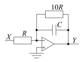
13: Filters Filters 1st Order Low-Pass Filter Low-Pass with Gain Floor **Opamp** filter Integrator  $\triangleright$  High Pass Filter 2nd order filter Sallen-Key Filter Twin-T Notch Filter **Conformal Filter** Transformations (A) **Conformal Filter** Transformations (B) Summary
