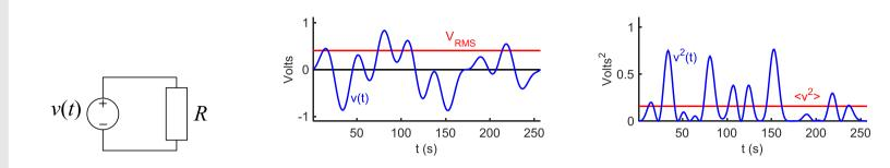
Intantaneous Power dissipated in R:  $p(t) = \frac{v^2(t)}{R}$
