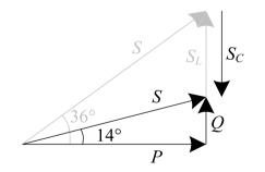
Average power to motor, P, is 10.6 kW in both cases.  $\left|\widetilde{I}\right|$ , reduced from  $56.5 \searrow 47 \text{ A} (-16\%) \Rightarrow \text{lower losses}$ . Effect of C: VARs =  $7.6 \searrow 2.6 \text{ kVAR}$ , power factor =  $0.81 \nearrow 0.97$ .
