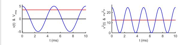
Cosine Wave:  $v(t) = 5 \cos \omega t$ . Amplitude is V = 5 V. Squared Voltage:  $v^2(t) = V^2 \cos^2 \omega t = V^2 \left(\frac{1}{2} + \frac{1}{2}\cos 2\omega t\right)$ Mean Square Voltage:  $\langle v^2 \rangle = \frac{V^2}{2}$  since  $\cos 2\omega t$  averages to zero. RMS Voltage:  $V_{rms} = \sqrt{\langle v^2 \rangle} = \frac{1}{\sqrt{2}}V = 3.54 \text{ V} = \widetilde{V}$
