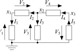
$= \sum_{n} \sum_{b} a_{bn} I_{b}^{*} x_{n} = \sum_{n} x_{n} \sum_{b} a_{bn} I_{b}^{*} = \sum_{n} x_{n} \times 0$ Note:  $\sum_{b} S_{b} = 0 \implies \sum_{b} P_{b} = 0$  and also  $\sum_{b} Q_{b} = 0$ .
