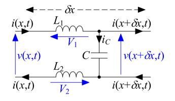
Capacitor equation:  $C\frac{\partial v}{\partial t} = i_C = i(x,t) - i(x + \delta x, t) = -\frac{\partial i}{\partial x}\delta x$ Inductor equation ( $L_1$  and  $L_2$  have the same current):  $(L_1 + L_2)\frac{\partial i}{\partial t} = V_1 + V_2 = v(x,t) - v(x + \delta x,t) = -\frac{\partial v}{\partial x}\delta x$ **Transmission Line Equations**
