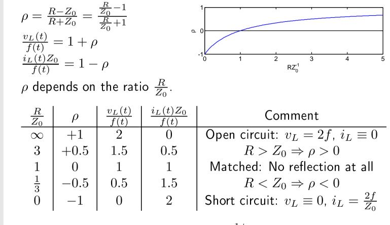
Note: Reverse mapping is  $R = \frac{v_L}{i_L} = \frac{1+\rho}{1-\rho} \times Z_0$ Remember:  $\rho \in \{-1, +1\}$  and increases with R.
