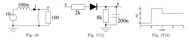
17. [E] In Fig. 17(i),  $v(t) = \begin{cases} 0 & t < 0 \\ 3 & 0 \le t < 1 \text{ ms} \text{ as shown in Fig. 17(ii). If the diode has a forward voltage} \\ 2 & t \ge 1 \text{ ms} \end{cases}$ drop of 0.7 V, find expressions for x(t) for  $t \ge 0$ .
