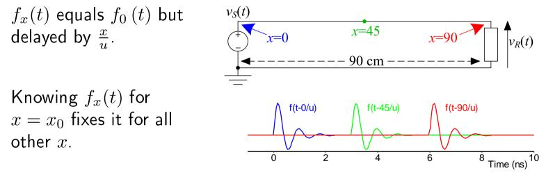
Backward wave:  $g_x(t)$  is the same but travelling  $\leftarrow: g_x(t) = g_0 \left(t + \frac{x}{u}\right)$ . Voltage and current are:  $v_x = f_x + g_x$  and  $i_x = \frac{f_x - g_x}{Z_0}$  where  $i_x$  is positive in the +x direction ( $\rightarrow$ ) and  $Z_0 = \sqrt{\frac{L_0}{C_0}}$
