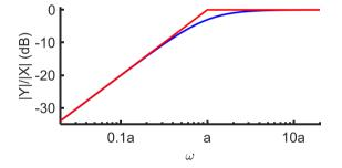
$$\frac{Y}{X} = \frac{R}{R+1/j\omega C} = \frac{j\omega RC}{j\omega RC+1} = \frac{j\omega RC}{\frac{j\omega}{a}+1}$$
