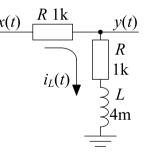
Sinusoidal input  $\Rightarrow$  Sinusoidal steady state  $\Rightarrow$  use phasors. Then convert phasors to time waveforms to calculate the actual output voltages  $y_{SS}(0-)$  and  $y_{SS}(0+)$  at t = 0. Revision Lecture 2: Transients & Lines Transients: Basic Ideas Steady States Determining Time ▷ Constant Determining Transient Amplitude Transmission Lines Basics Reflections Sinewaves and Phasors
