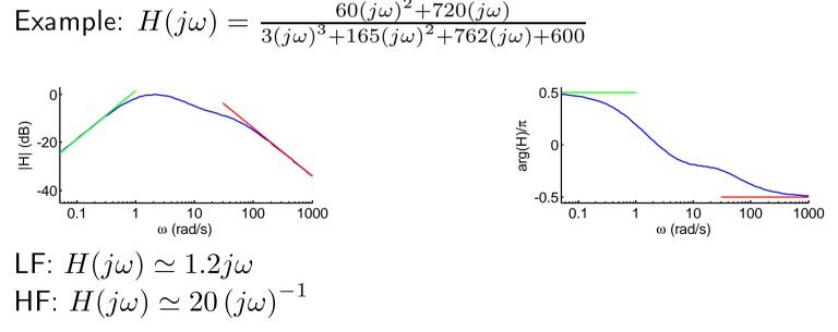
Revision Lecture 1: Nodal Analysis & **Frequency Responses** Exam Nodal Analysis **Op Amps Block Diagrams** Diodes **Reactive Components** Phasors **Plotting Frequency** Responses LF and HF Asymptotes **Corner frequencies**  $\triangleright$  (linear factors) Sketching Magnitude **Responses** (linear factors) Filters Resonance
