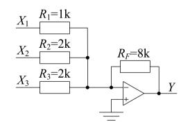
Nodal Analysis: Use two separate KCL equations at  $V_+$  and  $V_-$ . Do not do KCL at  $V_{out}$  except to find the op-amp output current.
