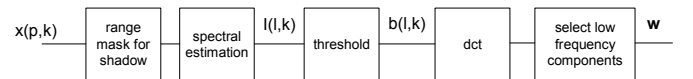
Fig.7 Procedure to calculate shadow features from HRR profiles using one of the three spectral estimation methods
