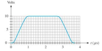
5. \*\* Determine the bit sequence represented by the waveform below. A bit period is 1µs. What is the total serial transfer time for the eight bits? What is the total parallel transfer time? Assuming that LSB is sent first, what is being transferred?
