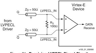
Figure 21: Receiving LVPECL Signal Circuit
