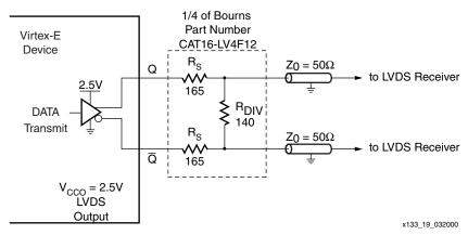
Figure 18: Transmitting LVDS Signal Circuit
