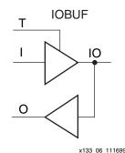
Figure 6: Input/Output Buffer Symbol (IOBUF
