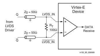
Figure 19: Receiving LVDS Signal Circuit
