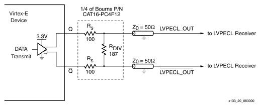
Figure 20: Transmitting LVPECL Signal Circuit
