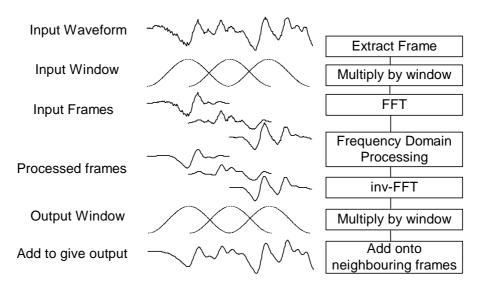
The output signal is thus formed by adding together a continuous stream of 256-sample frames each of which has been multiplied by both an input and an output window. If we choose the windows to be the square root of a Hamming window:
